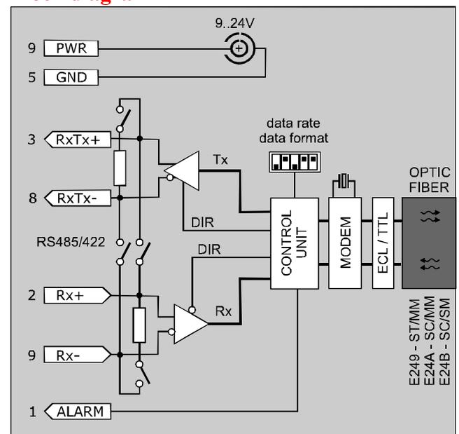
Modem ELO E245 is designed for singlemode fibers 9/125 μm. Its range is typically 15 km, optic connectors are SC type. For multimode cables 50/125 μm or 62.5/125 μm there are models ELO E244 with SC connectors and ELO E243 with ST ones.
