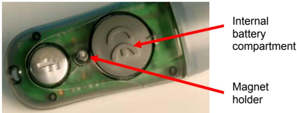
**Figure 2: MicroLite magnet holder**
