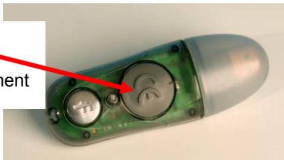
**Figure 1: MicroLite battery compartment**
